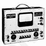
Here is an accurate tester that can keep up with you in your trouble-shooting work. Any one of its twenty scales is instantly connected to the test leads at the touch of a button! The vacuum tube voltmeter is stable and easy to use for checking AVC and AFC voltages, measuring oscillator output, amplifier gain, etc.
