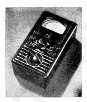
This is the new Model 023 circuit tester which is small enough to carry around in the pocket. The new tester does all the tricks of a larger unit and yet its size is only 5¼" long, 3" wide and 2¼" high.
